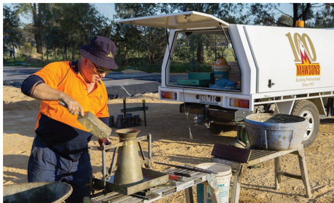
Preparing concrete samples for testing
